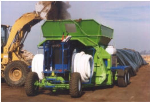
EcoPOD® with a 7 yard hopper, this system is powered with an 55 hp John Deere diesel engine and features a remote control unit to operate the hydraulics. This system can be used by a single operator and has a fill rate of 3+ tons per minute.
