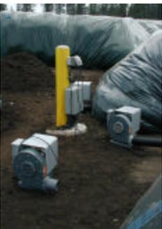
temperatures. Moisture is adjusted at time of filling or added to the total mixture upon blending. We maintain consistent moisture and temperature throughout the process while other systems do not. The compost matrix is sufficient in size to maintain heat, even in cold climates. Considered an in-vessel system, the Ag-Bag Environmental composting system is easily permitted.
