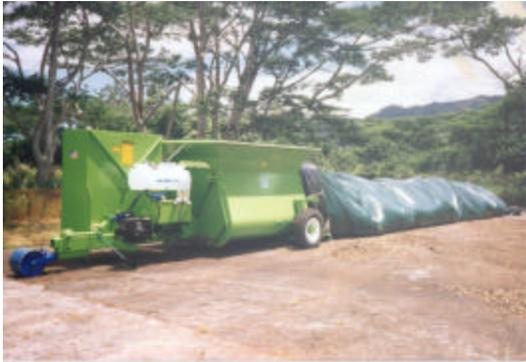
1-2 hours. This unit is small enough to tow down the road from site to site yet large enough to fit an industrial application. Powered with a 13 hp Honda engine (a diesel engine option is available) and features a remote control unit to operate the hydraulics. This system can be used by a single operator and has a fill rate of 1+ tons per minute.
