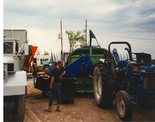
**Model CM-710** – This system uses a feed table conveyor that can be loaded with a front-end loader, rear unload or dump-trucks. Also using the 10' diameter x 200' length Eco-POD®, operations processing large quantities annually can best use this system. It is self-powered with a 120hp John Deere® engine and has wheel drive to move from EcoPOD® to EcoPOD®. The CM-710 has a fill rate of 3+ tons per minute.
