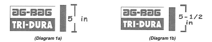
It is important to remember to keep the bag stretch mark between the 5 and 5-1/2 inches shown above. If you go under the 5 inch mark you will not get the proper use of you bag. If you go over the 5-1/2 inch stretch you risk causing damage to the bag.
