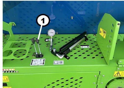
Figure 63. Conveyor Control Lever Key 1 – Conveyor Motor On/Off (Pull)
