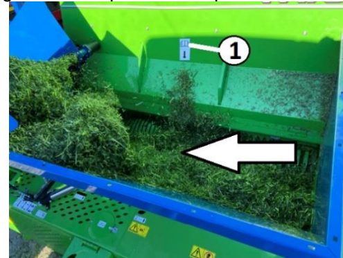
Figure 117. Optimum Crop Flow at Center Key 1 – Decal Location Arrow – Optimum Crop Flow Location
