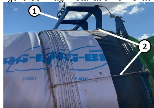
Figure 40. Bungee Retaining String (shown in final position for reference) Key 1–Bag Cradle Key 2–Strings (2 strings per side of bag cradle)
