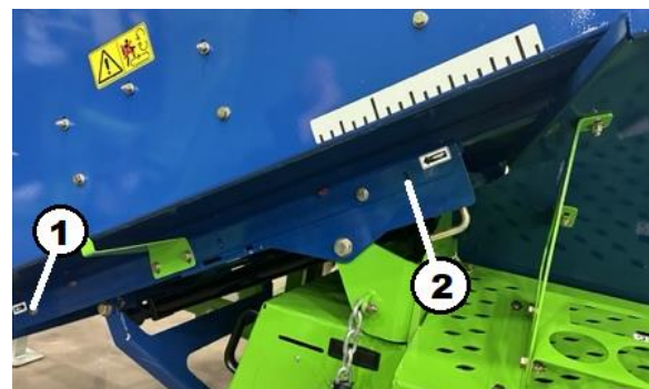
Figure 143. Conveyor Slide Greasing Key 1 – Lower Slide Grease Fitting Key 2 – Upper Slide Grease Fitting Note: Outer fittings shown. See back side for other 2 fittings.
