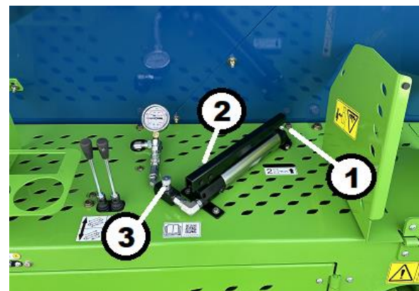
Figure 161. Brake System Hand Pump Key 1 – Fill Plug Key 2 – Pump Valve Key 3 – Needle Valve
