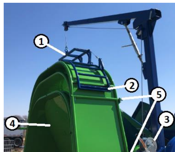
Figure 105. Bag Cradle Storage Key 1–Bag Cradle Key 2–Cradle Hook Key 3 – Winch Key 4 – Base Tunnel Key 5 – Storage Pin Locations
