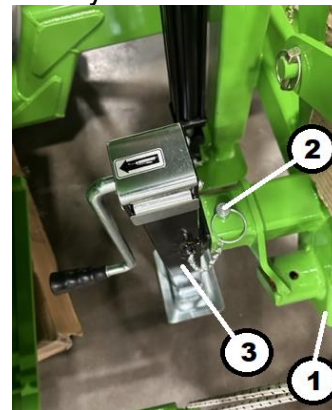
Fig. 90. Lift Jack Usage (T7170 Shown) Key 1 – Wheel Drop Key 2 – Cross Pin Key 3 – Lift Jack
