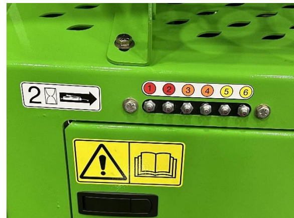
Figure 138. Grease Bank Key 1 and 2 – Rotor Bearings Key 3 and 4 – Jackshaft Bearings Key 5 and 6 – Distributor Bearings
