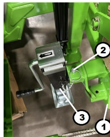
Fig. 27. Lift Jack Usage (T7170 Shown) Key 1 – Wheel Drop Key 2 – Cross Pin Key 3 – Lift Jack
