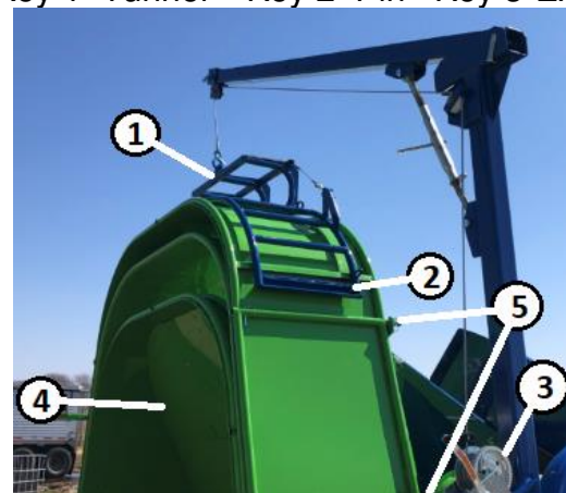
Figure 98. Tunnel Extension Lift Key 1–Bag Cradle Key 2–Cradle Hook Key 3 – Winch Key 4 – Base Tunnel Key 5 – Storage Pin Locations
