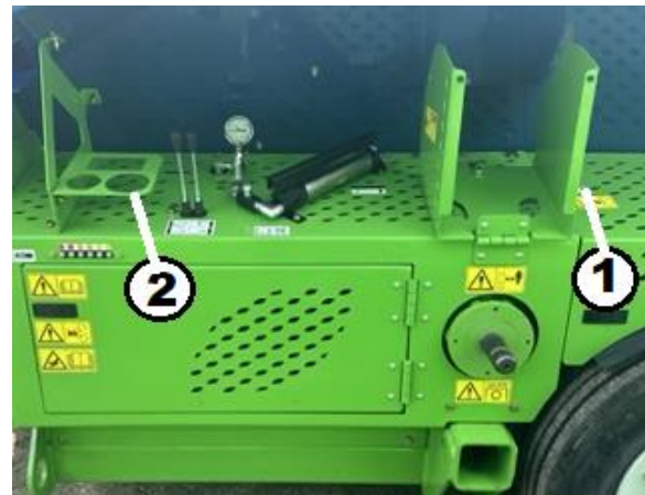
Fig. 149. Hyd. Pump Drive Chain Oiling Key 1 – Slot Key 2 – Bottle Storage
