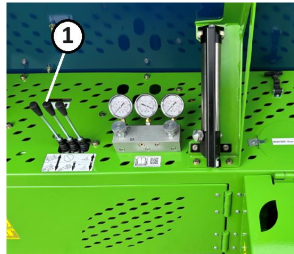
Figure 63. Conveyor Control Lever Key 1 – Conveyor Motor On/Off (Pull)
