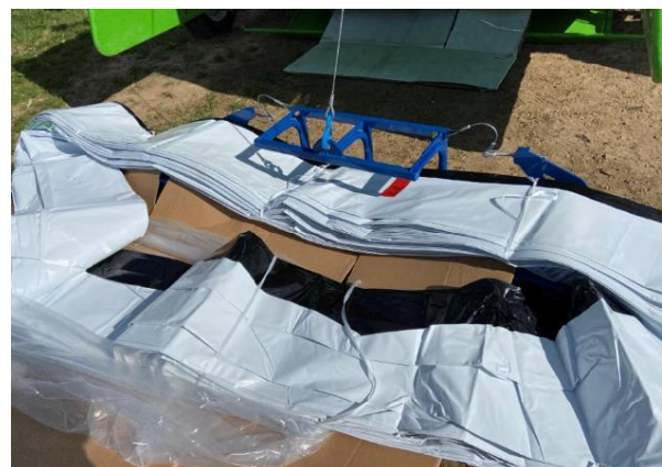
Figure 42. Bag Installation on Cradle
