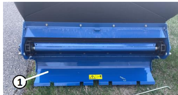
Figure 138. Conveyor Cleanout Open Key 1 – Conveyor Cleanout Door
