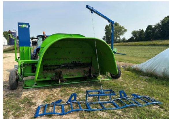
Figure 40. Cradle Lowered to Ground
