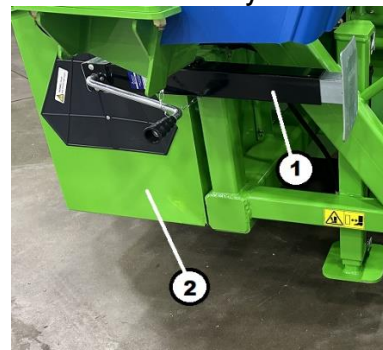
Figure 23. Lift Jack Storage (T7170) Key 1 – Lift Jack Key 2 – Storage (ref)
