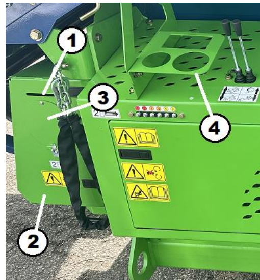
Figure 140. Rotor Drive Chain Oiling Key 1 – Oiling Slot Key 2 – Drive Cover Key 3 – Inspection Hole
