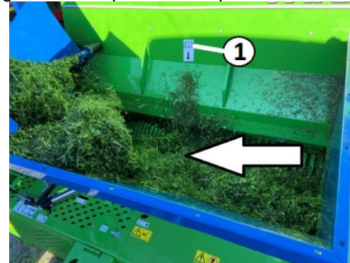
Figure 112. Optimum Crop Flow at Center Key 1 – Decal Location Arrow – Optimum Crop Flow Location
