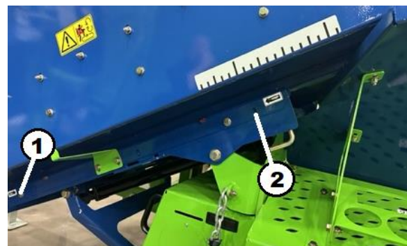
Figure 136. Conveyor Slide Greasing Key 1 – Lower Slide Grease Fitting Key 2 – Upper Slide Grease Fitting Note: Outer fittings shown. See back side for other 2 fittings.
