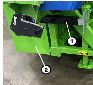
Figure 93. Lift Jack Storage (T7170) Key 1 – Lift Jack Key 2 – Storage (ref)
