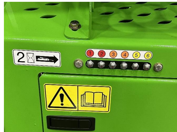
Figure 133. Grease Bank Key 1 and 2 – Rotor Bearings Key 3 and 4 – Jackshaft Bearings Key 5 and 6 – Distributor Bearings
