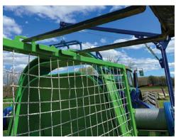
**Redesigned Backstop Lifting Points** Backstop can be lifted with multiple devices without getting close to rope webbing.
