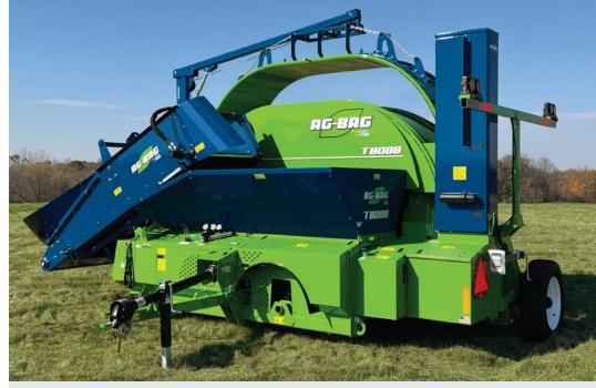
The mighty T8088 Ag-Bagger features the industry's widest 104-inch revolutionary rotor with 156 teeth resulting in the best forage flow, highest unload rates, and most-dense packing in a 10-foot or 12-foot tunnel and up to 500-foot long Ag-Bags.
