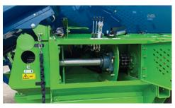
**Operator Station with Serviceability** Operators can easily adjust the conveyor, conveyor lift, cable rewind and brake pressure with easy to access controls. Serviceability features are located in this same area. Operators can grease all bearings with a central grease bank, oil chain drives, and store chain lubes. PTO holder for quick removal is located here too.
