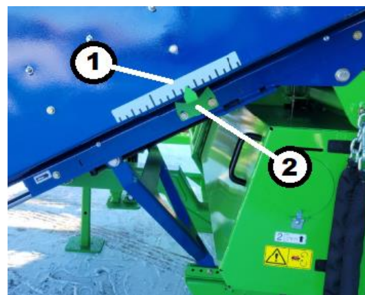
Figure 114. Conveyor Position Key 1 – Ruler Decal Key 2 – Marker
