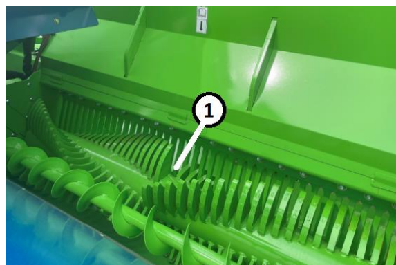
Figure 62. Stripper Plate Visual Check Key 1 – Visual Check
