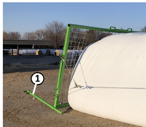
Figure 65. Support Feet Removal Key 1 – Support Feet
