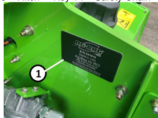
Figure 11. S/N Tag Location (inside compartment) Key 1 – S/N Tag
