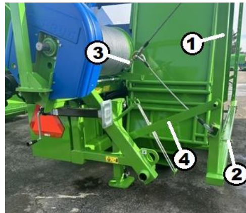
Figure 103. Backstop Storage Position Key 1 – Backstop Key 2 – Pin Key 3 – Backstop Sling and Cable Key 4 – Stabilizer Arm
