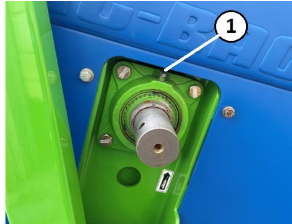
Figure 139. Cable Drum Bearing Key 1 – Grease Fitting
