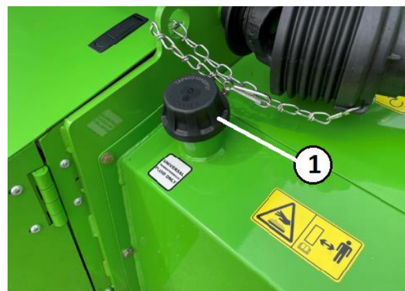
Fig. 153. Vented Hyd. Reservoir Cap Key 1 - Cap
