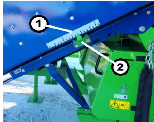
Figure 115. Conveyor Position Key 1 – Ruler Decal Key 2 – Marker
