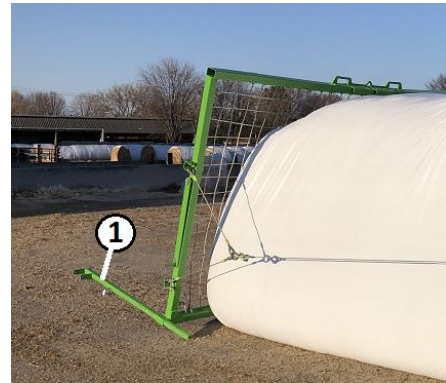
Figure 71. Support Feet Installation Key 1 – Support Feet
