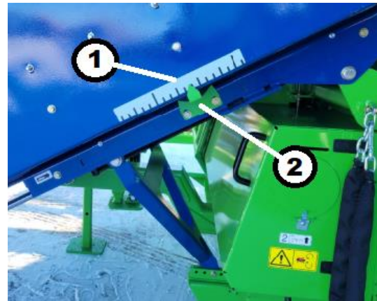
Figure 82. Conveyor Lift Lock Key 1 – Lock Lever Key 2 – Marker
