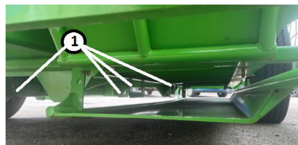
Figure 176. Bottom View from Bag Pan Key 1 – Fork Pockets
