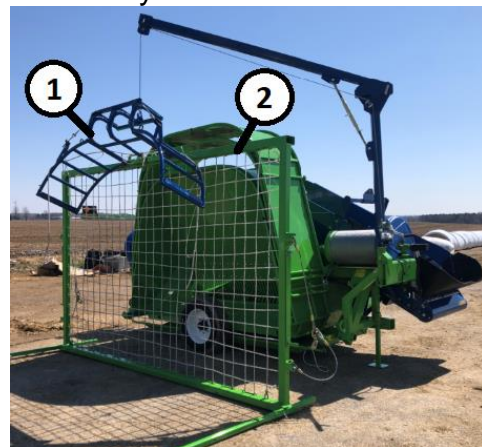
Figure 101. Backstop with Cradle Key 1 – Cradle Key 2 - Backstop
