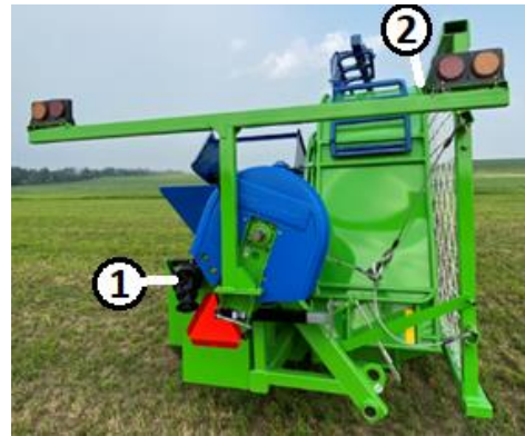
Figure 109. Narrow Transport Key 1 – PTO Rear Storage Key 2 – Narrow Storage Positions
