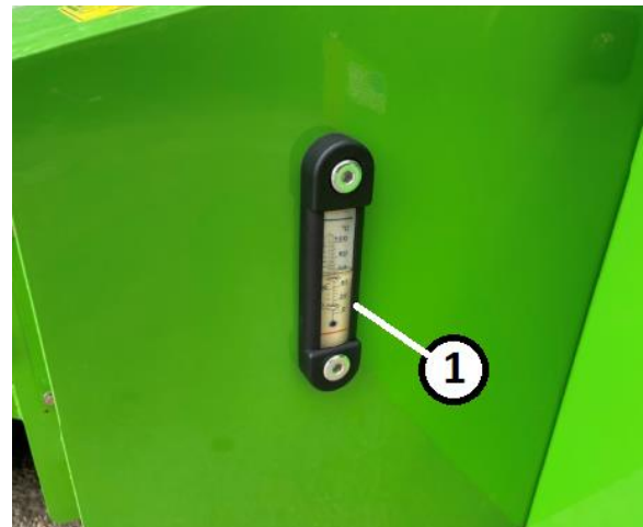
Fig. 152. Hydraulic Oil Reservoir Level Key 1 – Hyd. Oil Level Gauge
