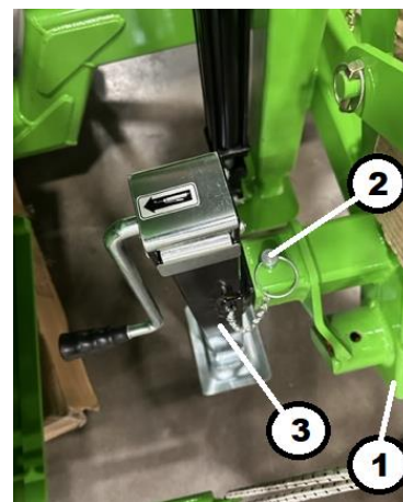
Fig. 21. Lift Jack Usage Key 1 – Wheel Drop Key 2 – Cross Pin Key 3 – Lift Jack
