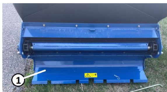
Figure 145. Conveyor Cleanout Open Key 1 – Conveyor Cleanout Door
