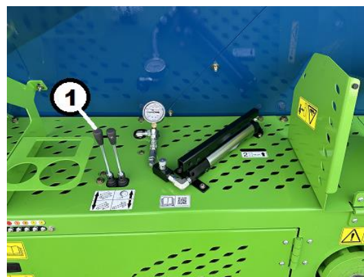
Figure 119. Conveyor Raise and Lower Key 1 – Control Lever
