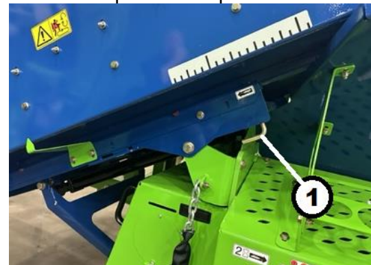
Figure 118. Conveyor Lift Lock Key 1 – Lock Lever
