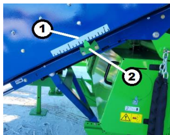
Figure 55. Conveyor Position Key 1 – Ruler Decal Key 2 – Marker
