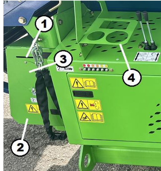
Figure 146. Rotor Drive Chain Oiling Key 1 – Oiling Slot Key 2 – Drive Cover Key 3 – Inspection Hole Key 4 – Bottle Storage
