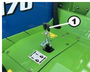
Figure 22. Operator Controls Key 1 – Machine Lift / Lower Lever
