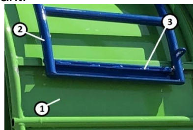
Figure 33. Cradle Hook Key 1–Ext. Key 2–Cradle Key 3–Hook
