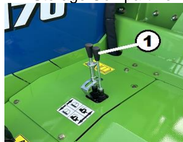
Figure 92. Operator Controls Key 1 – Machine Lift / Lower Lever
