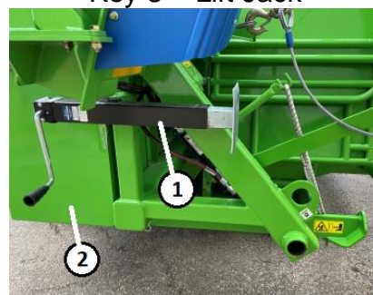
Figure 91. Lift Jack Storage (T7170) Key 1 – Lift Jack Key 2 – Storage Compartment (ref)
