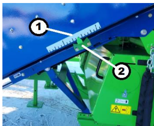
Figure 64. Conveyor Position Key 1 – Ruler Decal Key 2 – Marker
