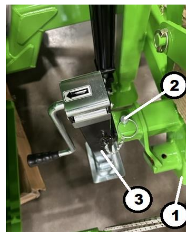
Fig. 84. Lift Jack Usage (T7170 Shown) Key 1 – Wheel Drop Key 2 – Cross Pin Key 3 – Lift Jack
