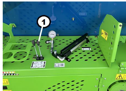
Figure 72. Brake System Control Key 1 – Cable Rewind Control
