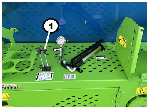
Figure 63. Conveyor Control Lever Key 1 – Conveyor Motor On/Off (Pull)
