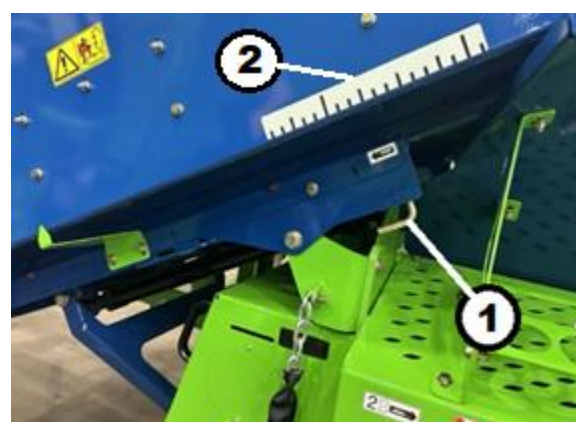
Figure 120. Conveyor Position Key 1 – Ruler Decal Key 2 – Marker
