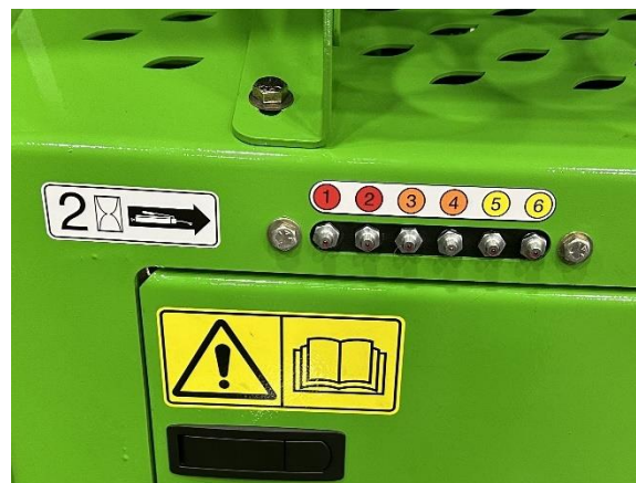
Figure 138. Grease Bank Key 1 and 2 – Rotor Bearings Key 3 and 4 – Jackshaft Bearings Key 5 and 6 – Distributor Bearings
