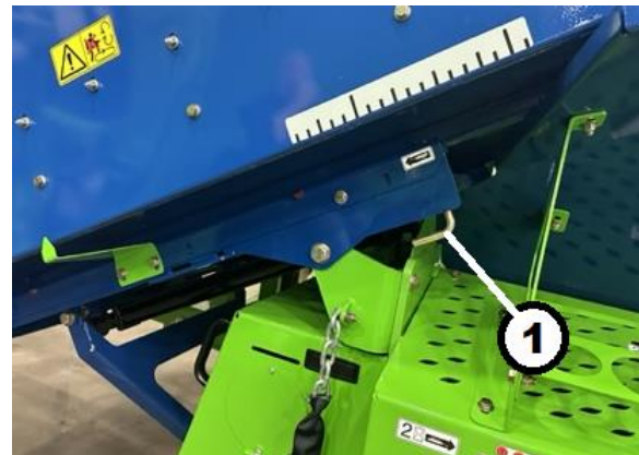
Figure 53. Conveyor Lift Lock Key 1 – Lock Lever
