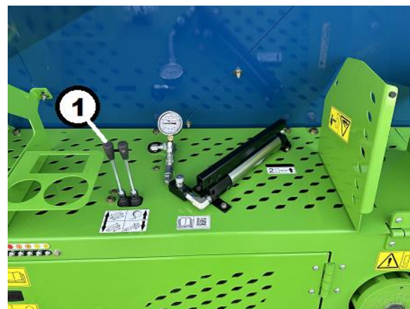
Figure 54. Conveyor Raise and Lower Key 1 – Control Lever
