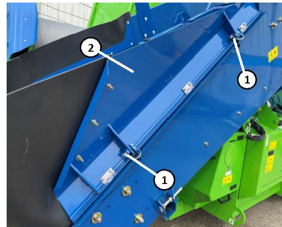
Figure 110. Conveyor Extension Key 1 – Lynch Pins Key 2 – Extension
