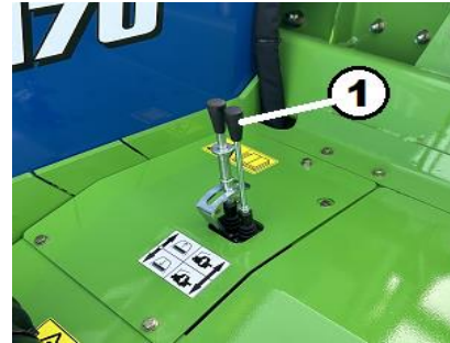
Figure 85. Operator Controls Key 1 – Machine Lift / Lower Lever
