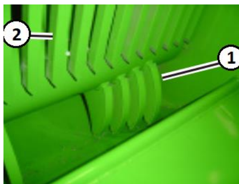
Figure 162. Rotor Tooth Tine Cap Key 1 – Cap Installed Key 2 – Stripper Bar Plate
