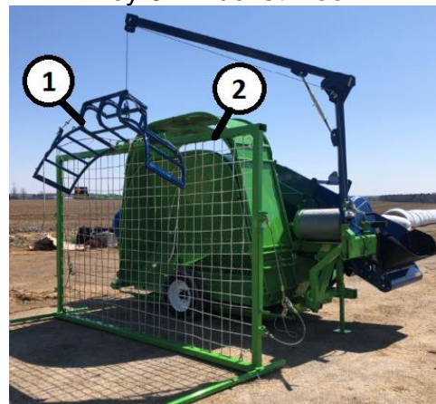
Figure 15. Backstop with Cradle Key 1 – Cradle Key 2 - Backstop
