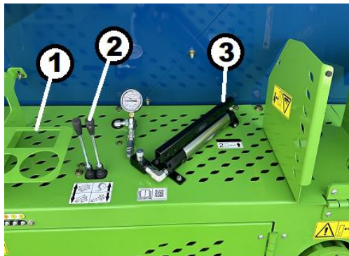
Figure 10. Operator Station Key 1–Oil Storage Key 2 - Control Levers Key 4 - Brake Hand Pump
