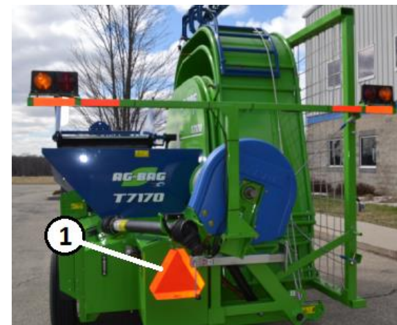
Figure 186. SMV Installation Key 1 – SMV Sign
