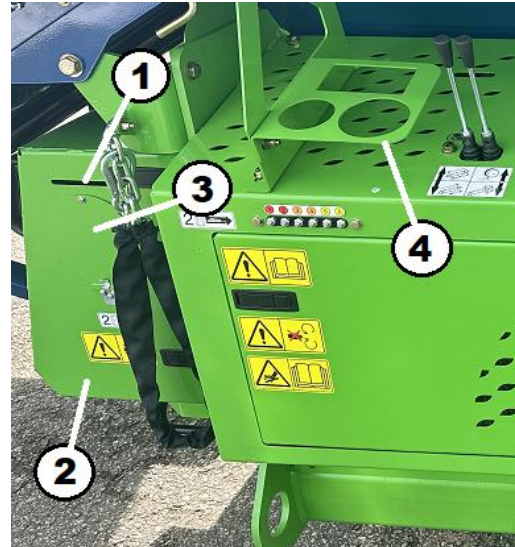
Figure 140. Rotor Drive Chain Oiling Key 1 – Oiling Slot Key 2 – Drive Cover Key 3 – Inspection Hole
