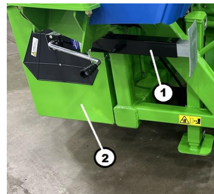
Figure 85. Lift Jack Storage Key 1 – Lift Jack Key 2 – Storage Compartment (ref)
