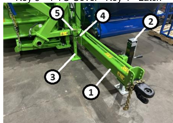
Figure 97. Hitch in Transport Position Key 1 – Hitch Key 2 – Lift Jack Key 3 – Jack Stand Key 4 – Hitch Cross Pin Key 5 – Jack Stand Cross Pin
