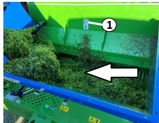
Figure 108. Optimum Crop Flow at Center Key 1 – Decal Location Arrow – Optimum Crop Flow Location
