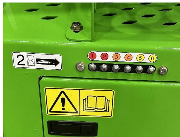
Figure 133. Grease Bank Key 1 and 2 – Rotor Bearings Key 3 and 4 – Jackshaft Bearings Key 5 and 6 – Distributor Bearings
