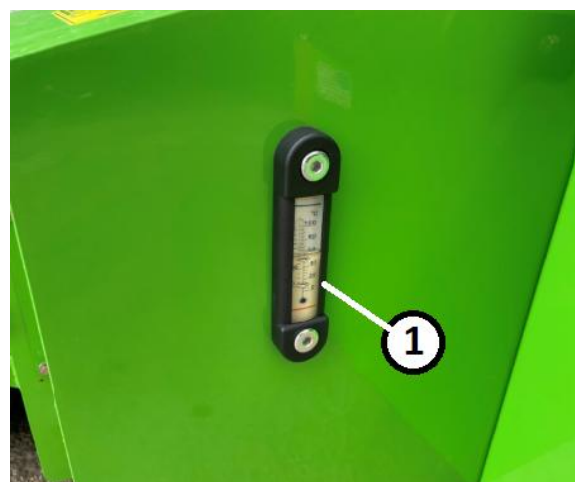
Fig. 149. Hydraulic Oil Reservoir Level Key 1 – Hyd. Oil Level Gauge (1/2 full)
