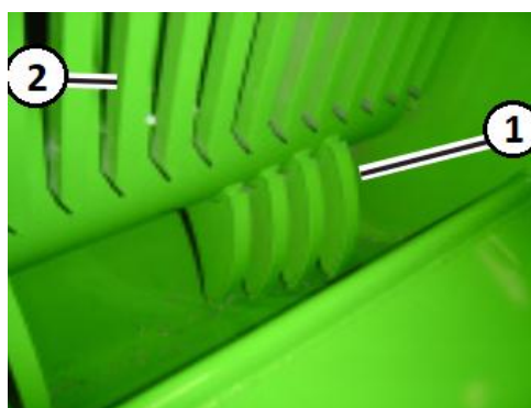
Figure 156. Rotor Tooth Tine Cap Key 1 – Cap Installed Key 2 – Stripper Bar Plate
