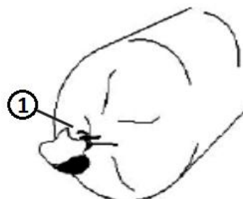
Figure 48. Start of Double-Knot Tie Key 1 – First Tie
