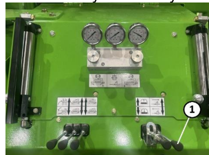
Figure 33. Anchor Position Control Key 1 – Control
