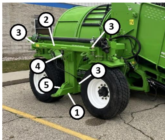
Figure 13. Retracted Transport Hitch Key 1 – Hitch Key 2 – Brace Key 3 – Pin + Clip Key 4 – Harness Key 5 – Safety Chain
