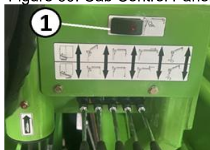
Figure 61. Bag Boom Light Switch Key 1 – Light Switch
