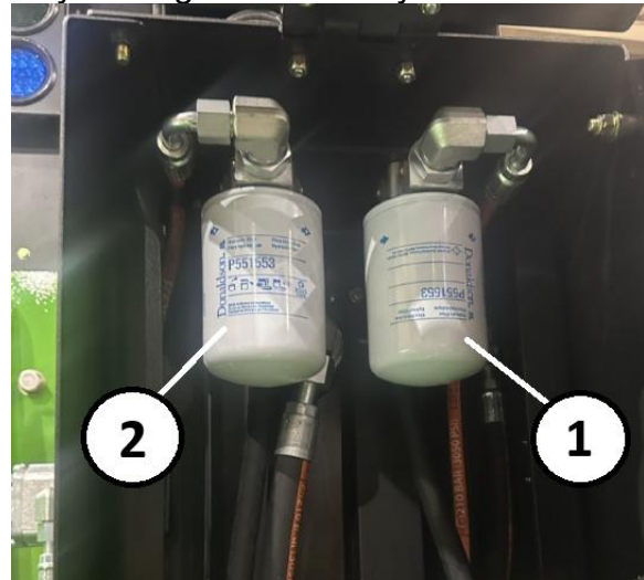
Figure 123. Filters Key 1 – Planetary Filter Key 2 – Gearbox Filter
