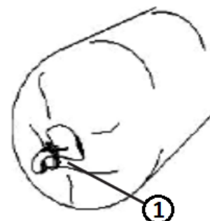
Figure 49. End of Double-Knot Tie Key 1 – Fold Over and Second Tie
