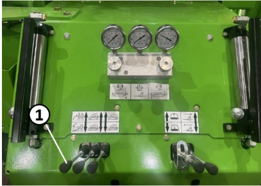
Figure 22. Operator Station Key 1 – Feedtable Raise/Lower Control
