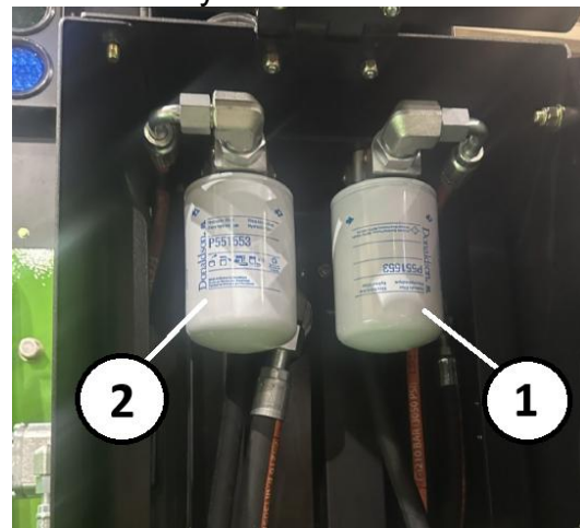
Figure 123. Filters Key 1 – Planetary Filter Key 2 – Gearbox Filter
