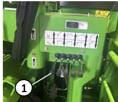
Figure 36. Bag Pan Control Key 1 – Bag Pan Control Lever
