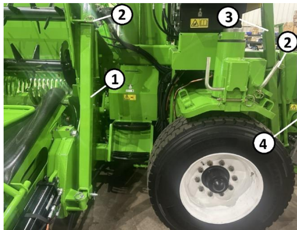
Figure 84. Hitch and PTO Storage Key 1 – Hitch Brace Storage Key 2 – Lock Bracket, Pin and Clip Key 3 – Hitch Key 4 – PTO (PTO stored vertically – reference only)
