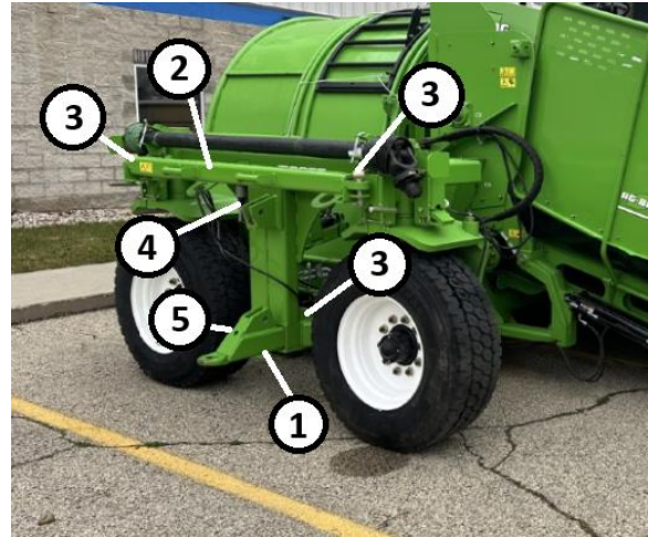
Figure 85. Retracted Transport Hitch Key 1 – Hitch Key 2 – Brace Key 3 – Pin + Clip Key 4 – Harness Key 5 – Safety Chain
