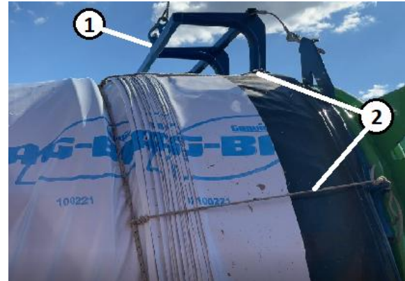
Figure 41. Bungee Retaining String (shown in final position for reference) Key 1–Bag Cradle Key 2–Strings (2 strings per side of bag cradle)
