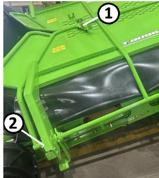
Figure 75. Wing Latches Key 1 – Transport Latch Key 2 – Ag-Bagging Latch
