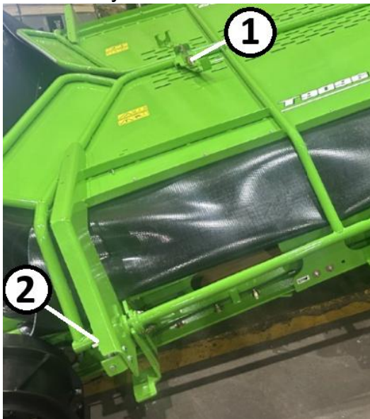
Figure 24. Wing Latches Key 1 – Transport Latch Key 2 – Ag-Bagging Latch
