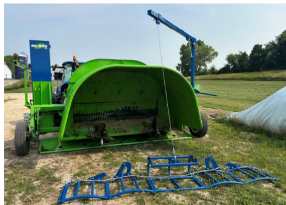
Figure 38. Cradle Lowered to Ground
